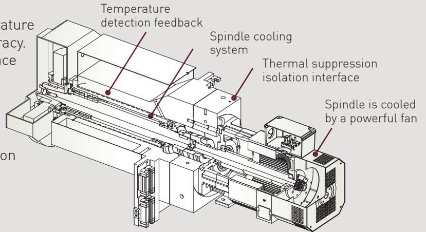
The machine's powerful spindle provides greater accuracy and precision for superior cutting efficiency
