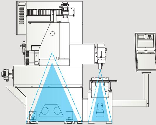
To prevent vibration and ensure machining accuracy, the high-strength rigid design is built to withstand the maximum force caused by deformation.
