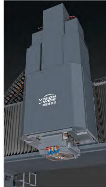
4 corners of the slide rail are supported on 8 sides
