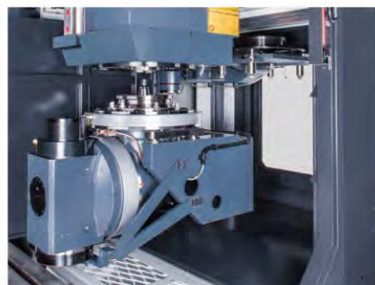
● Auto swiveling arm type head bracket (on operation side)
