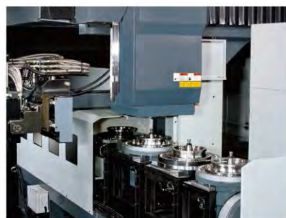
● Multi-heads magazine(magazine side)
