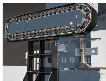
● Floor-standing vertical type tool magazine(opt.)
