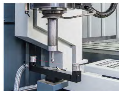
● Tool length measurement device at magazine side for mold cutting to change tool fast.(opt.)
