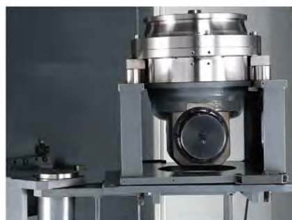
● Manual swiveling arm type head bracket(on operation side)
