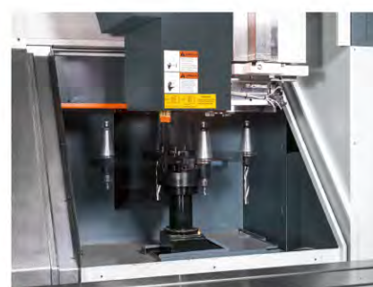
● Auto tool exchange, tool to tool 3 sec. in vertical type
