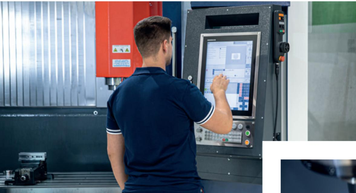
The EMCOMILL is equipped with state-of-the-art control technology, either Siemens 828D with ShopMill, Heidenhain TNC 620 or Fanuc Oi-MF with Manual Guide i are available. The control panel includes a swivel function for an ergonomic working position.
