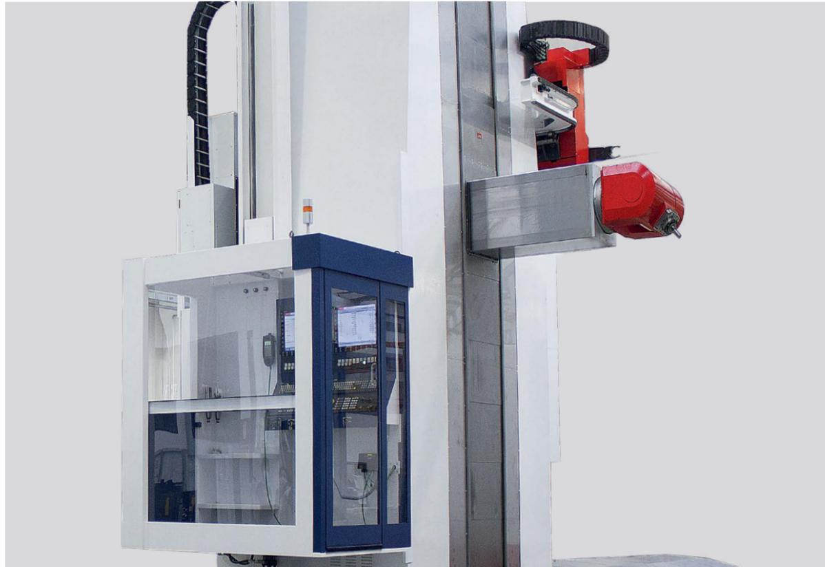
POMO and POVT Operator platform with vertical (up to 2500 mm) and cross travel (up to 800 mm).
