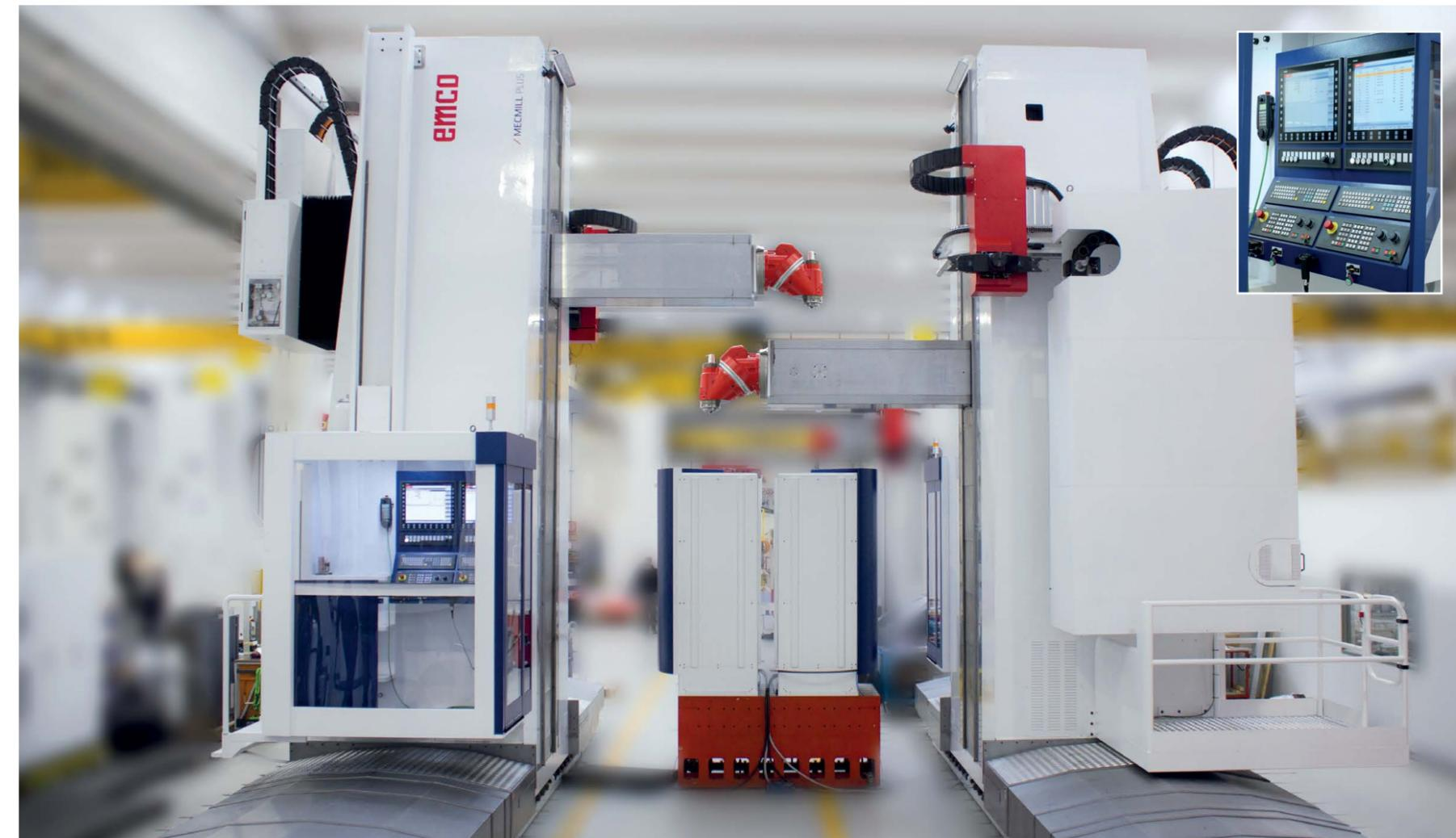
Opposite machines - Master and slave machine with master and slave CNC. The milling center is equipped with SANT-anticollision software.
