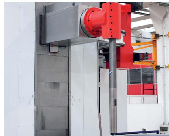
Turning head for supporting a special boring bar: 120 mm diameter, length up to 1500 mm for turning operations up to 1000 mm depth.
