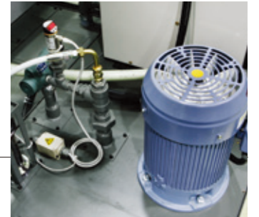
Spindle-through coolant 3MPa
