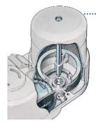
The TMV is the only mill in its class that uses a roller bearing for the lower support of the motor shaft. It ensures proper loading, support, and alignment for quiet, accurate operation at any speed. It also prevents the shaft from being distorted by the tension of the belt over years of use.
