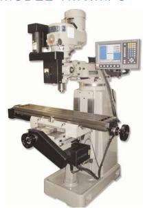
Acu-rite Millpower CNC Control 10" x 50" Table, 15.5" x 31" Travel, 3 hp Spindle Motor, 60 - 4,500 rpm Variable Speed Drive
