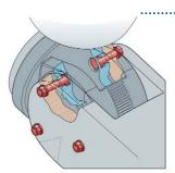
This patented knuckle-head design prevents the head from slipping. Sharp mills have a knuckle which uses 6 bolts, 3 per side, fitted into circular T-slots with nuts securing them from the outside. This method locks the head into place more securely resulting in better accuracy and performance.
