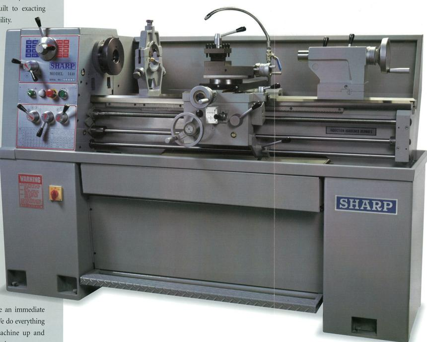
They may look small, but the 1340F and 1440F cut like no small lathe you've ever seen. Both have an extra-wide 8.5" bed way, a larger apron, compound and a generous 13.5" cross slide. The result is lathes which perform even heavy cuts with pinpoint precision and accuracy.
