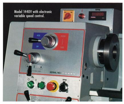
It takes just a turn of the RPM control knob to change speeds on our model 1440V lathe. The electronic variable speed control utilizes a frequency drive inverter to change motor speeds, while the high/low gear design ensures power in the lower speed range.
