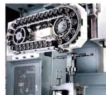
● Vertical type tool magazine to save floor space, 40 tools magazine (60 tools opt.)
