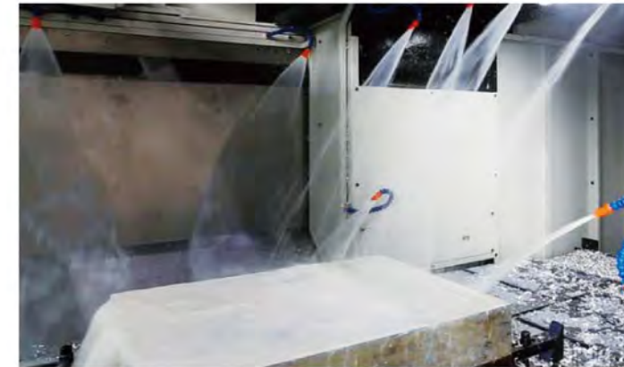
● Water fall flushing system (Opt.) Chip clean flushing device under the beam
