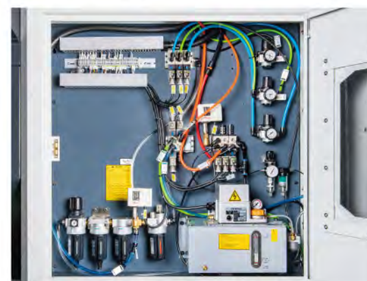
● Centralized auto lubrication system
