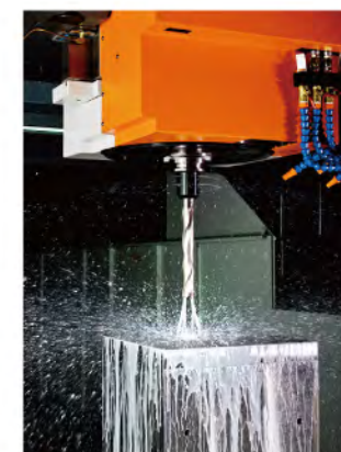
● Coolant through spindle (Opt.)
