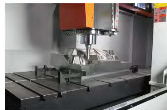
● Horizontal T-slots on work table for quick positioning and mold clamping
