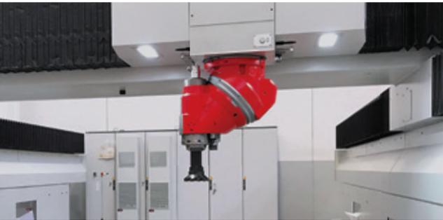
Z-axis saddle integrated in the machine crossbeam, its structure ensures highest stiffness results and utmost dynamic.
