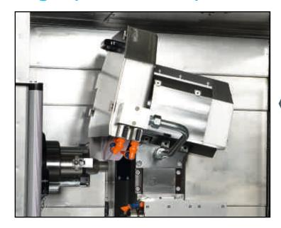
External grinding with powerful grinding spindle in angular plungecut, also suitable for face grinding of shoulders.
