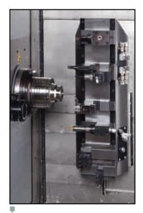
**L-Version**Spindle with high precision positioning in X1/Z1 and linear tooling as optimal rigid hard-turning and micro-finishing machine
