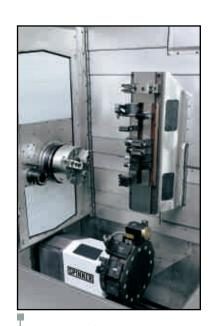
**LT-Version**With additional turret with driven tools and Y1 axis in the lower part of the workspace
