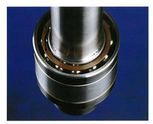
A matched pair of super-precision ABEC-7 angular contact bearings support the spindle. The quill is CNC-ground to a mirror finish, then chromed to fit the housing. Together, they insure spindle runout of no more than 0.0002" T.I.R.—a tolerance unsurpassed in the industry.
