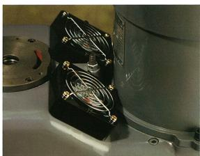
A pair of high-output fans keep the LMV's powerful 3 h.p. head cool—one of a series of heat-dispersion features that allow the LMV to work demanding jobs for extended periods without damaging the motor, belts or bearings.
