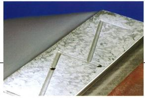
The underside of the saddle is hand-scraped for better oil retention. Our craftsmen repeatedly match the surfaces of each unit and check for precise fit, to guarantee more complete oil retention. This extra step avoids having chips and dirt embed in the knee and damage the sliding surface.
