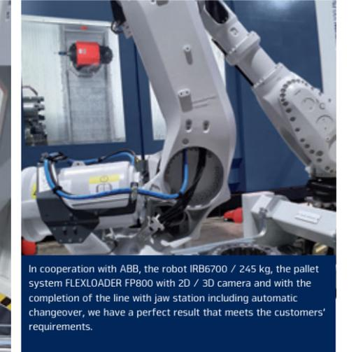
In cooperation with ABB, the robot IRB6700 / 245 kg, the pallet system FLEXLOADER FP800 with 2D / 3D camera and with the completion of the line with jaw station including automatic changeover, we have a perfect result that meets the customers' requirements.
