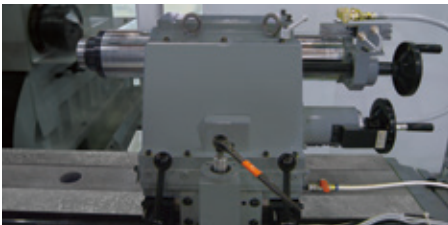
The photo is of a footstock with 1,000kg specifications
