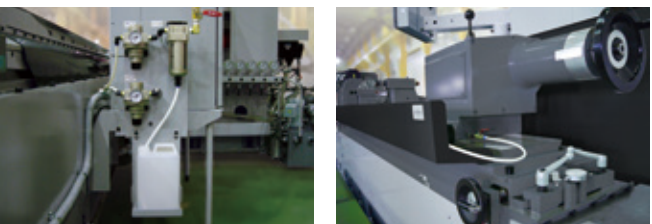
The photo is of a footstock with 1,000kg specifications
