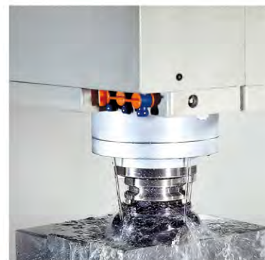
● Fluid nozzle for spindle provides best spray angle. (not available for head attachment)
