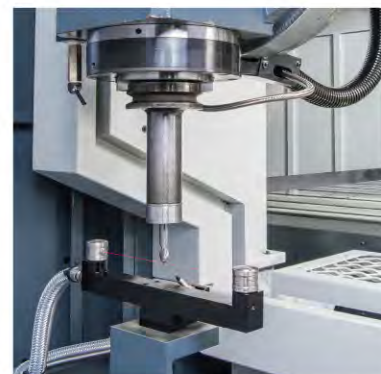
● Tool length measurement device at magazine side for mold cutting to change tool fast.
