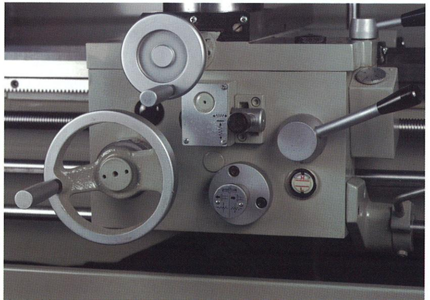
The apron is equipped with a push-pull knob that controls the feed direction of the carriage. It is also equipped with a clutch that protects the feed mechanism in the event of overload.
