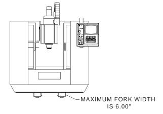
Figure 3-2 Moving the VMC
