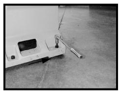
Figure 3-19 Drive Down Corner Leveling Screws
