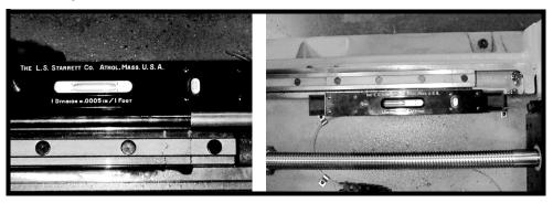
Figure 3-21 Take Leveling Measurements (6535 on right).
