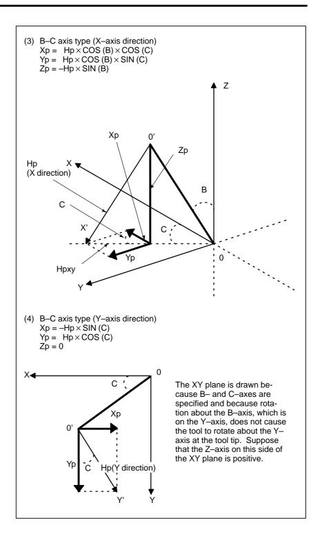
In the figures above, a, b, and c represent the positions (angles) of the A-axis, B-axis, and C-axis from the machine zero point; those values present when the tool axis direction handle feed mode is set or a reset occurs are used. To change the feed direction, reenter the tool axis direction handle feed mode, or press the reset key.
