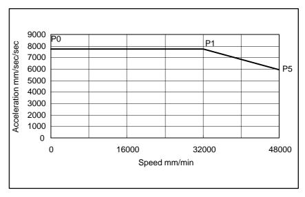
Fig.19.10 (f) Acceleration pattern with consideration of friction
