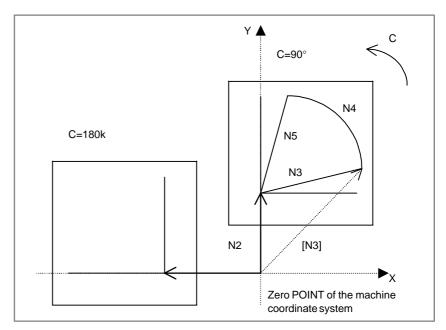
Fig.14.14 (b) Example of fixture offset
