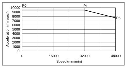
Fig.19.10(I) Acceleration pattern in case of – move and acceleration
