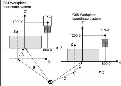
X' - Z' - New workpiece coordinate system
