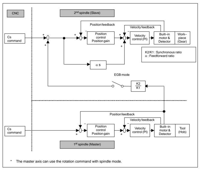
Fig. 20.8.3 (a) Block diagram for Spindle EGB control
