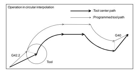
Fig. 22.5.1 (b) Operation at compensation start-up and cancellation (Type A)
