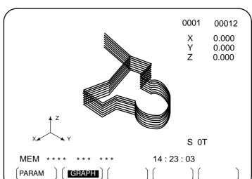
**6** Automatic operation is started and machine movement is drawn on the screen.
