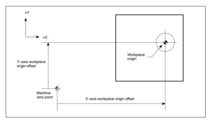
In the above case, the workpiece origin is located at the center of a hole in the workpiece. A measurement probe having a sensor at its tip is used to measure the positions of three arbitrary points on the circumference of the hole. The three points prescribe a unique circle, the center of which is set as the X-/Y-axis workpiece origin. Set bit 4 (WMH) of parameter No. 5007 to 1 before starting the measurement.
