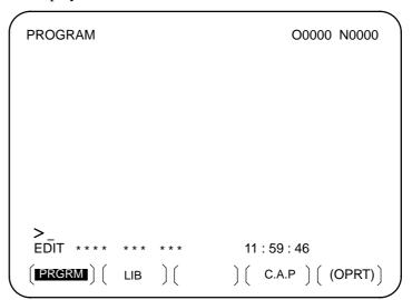
3 Key in the program number of a program to be registered after keying in address O, then press [INSERT]. For example, when a program with program number 10 is to be registered, key in O 1 0, then press [INSERT]. This registers a new program O0010.
