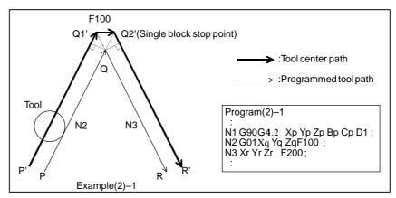
Fig. 22.5.1 (g) Operation in the compensation mode (2)
