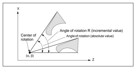
Fig. 14.10 (b) Coordinate system rotation
