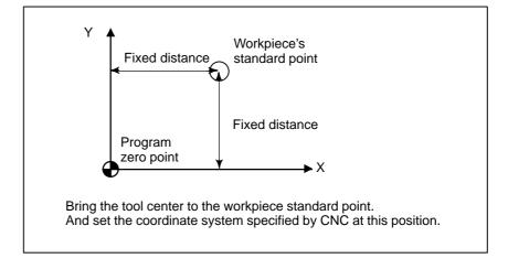
(2) Mounting a workpiece directly against the jig
