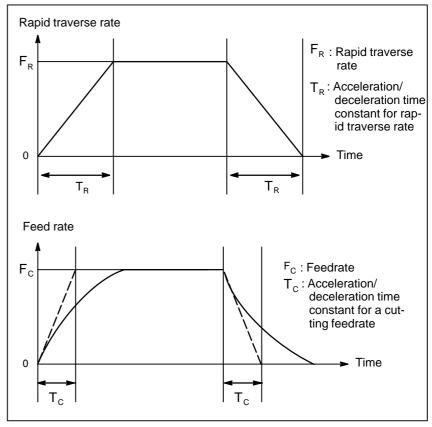
Fig. 5.1 (a) Automatic acceleration/deceleration (example)
