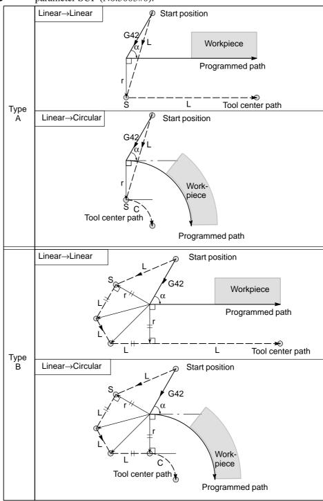
Tool movement around the outside linear→linear at an acute angle less than 1 degree (α<1°)</li>
