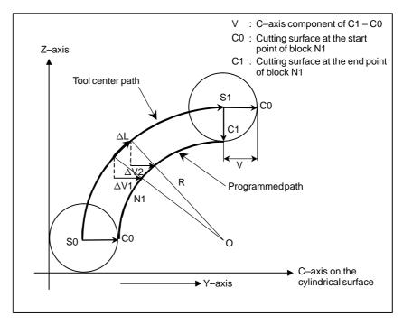
Fig. 22.2 (c) Cutting Point Compensation in a Circular Command Block
