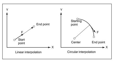
Fig. 5.3 (a) Tangential feedrate (F)
