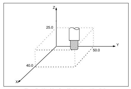
Fig. 7 Tool Position Specified by X40.0Y50.0Z25.0
