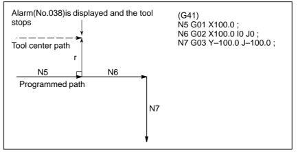
Change in the offset direction in the offset mode The offset direction is decided by G codes (G41 and G42) for cutter radius and the sign of cutter compensation value as follows.
