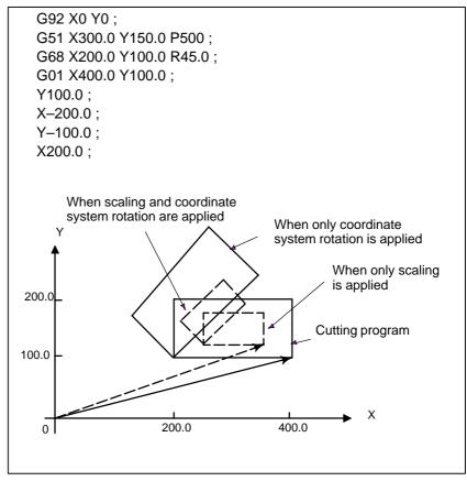
Fig. 14.10 (e) Scaling and coordinate system rotation in cutter compensation C mode
