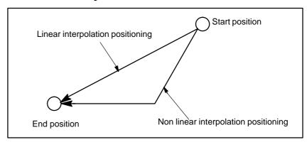
The rapid traverse rate in G00 command is set to the parameter No. 1420 for each axis independently by the machine tool builder. In the positioning mode actuated by G00, the tool is accelerated to a predetermined speed at the start of a block and is decelerated at the end of a block. Execution proceeds to the next block after confirming the in–position.
