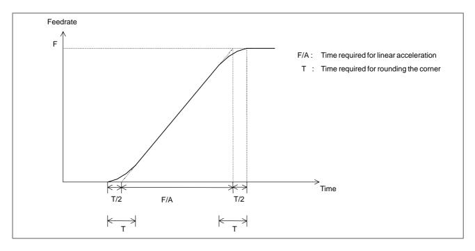
When the non-linear interpolation type is selected, movement is performed at the feedrate set in parameter No. 1420 with acceleration/deceleration set in parameter No. 1620. The corresponding value can be set in parameter No. 1621 to select bell-shaped acceleration/deceleration. (To select bell-shaped acceleration/deceleration, the option of bell-shaped acceleration/deceleration for rapid traverse is required.)
