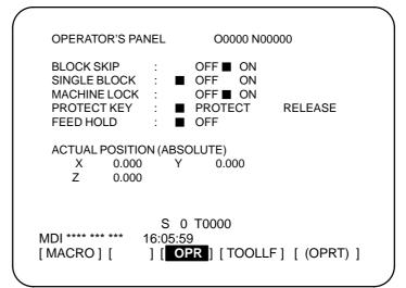
4 Move the cursor to the desired switch by pressing cursor key or .
