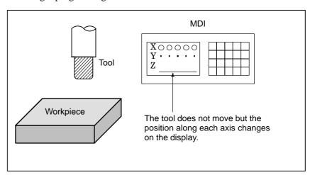
Fig. 5.1 Machine lock
