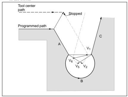
After ignoring vectors  $V_2$  and  $V_5$  because of interference, interference also occurs between vectors  $V_1$  and  $V_6$ . The alarm is displayed and the tool is stopped.
