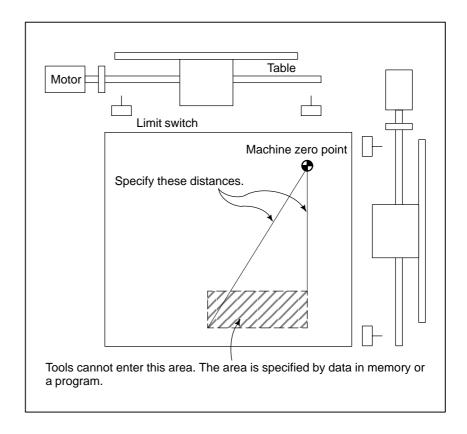
Besides strokes defined with limit switches, the operator can define an area which the tool cannot enter using a program or data in memory. This function is called stroke check (see III–6.3).
