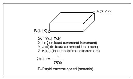
Fig. 6.3 (c) Creating or changing the forbidden area using a parameters
