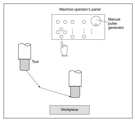
Fig. 1.1 (b) The tool movement by manual operation
