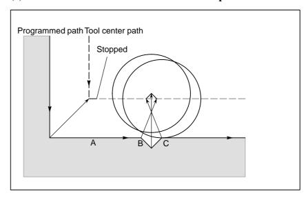
Like (1), P/S alarm is displayed because of the interference as the direction is reverse in block B.
