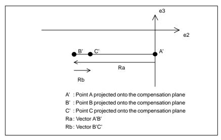
Fig. 22.5.1 (r) Programmed Path (on the Compensation Plane) before and after the End Point (Point B) of N4
