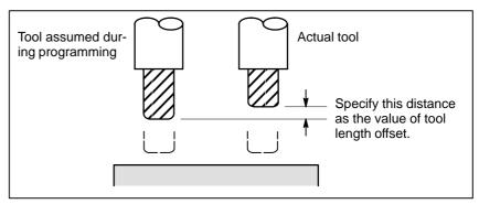
Fig. 14.1 Tool length offset
