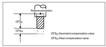
Fig. 14.8 (a) Geometric compensation and wear compensation
