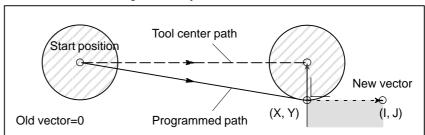
Unless otherwise specified, (I, J) are assumed to be equal to (X, Y). When the following command is specified, a vector perpendicular to a line connecting the start position and position (X, Y) is created.
