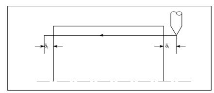
Fig. D.2 (a) Incorrect threaded portion
