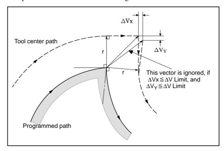
If  $\Delta Vx \le \Delta V$  limit and  $\Delta Vy \le \Delta V$  limit, the latter vector is ignored. The  $\Delta V$  limit is set in advance by parameter (No. 5010).
