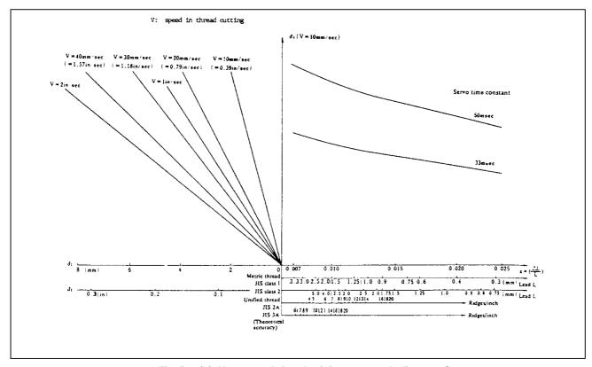
Fig. D.2 (b) Nomograph for obtaining approach distance  $\delta_{\text{1}}$
