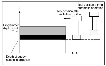
Fig. 1.3 (c) Handle Interruption for Automatic Operation
