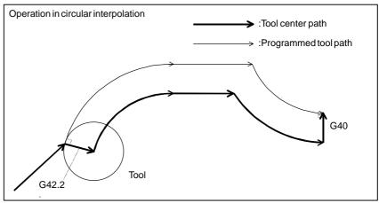
Fig. 22.5.1 (d) Operation at compensation start-up and cancellation (Type C)
