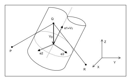
Fig. 22.5.1 (j) Compensation vector calculation
