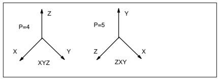
Fig. 12.2.1 (a) Coordinate systems for the isometric projection
