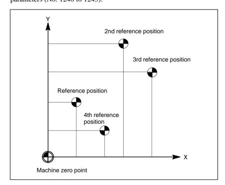
Fig. 6.1 (a) Machine zero point and reference positions
