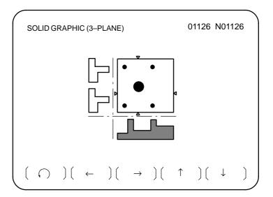
17 Each time soft key [ ) is pressed, the side–view drawings displayed change as follows.
