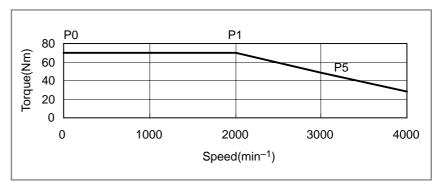
Fig.19.10(g) Torque for Acc/Dec in case of + move and acceleration
