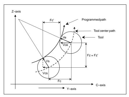
Fig. 22.2 (h) Actual Speed Indication during Circular Interpolation
