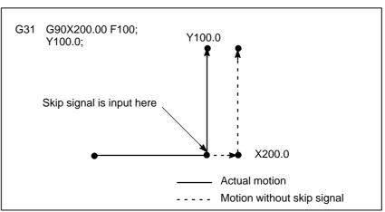
Fig. 4.16 (b) The next block is an absolute command for 1 axis
