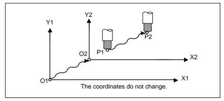
Fig. 3.5 (b) Coordinates with the switch OFF
