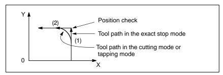
Fig. 5.4.1 (a) Example of Tool Paths from Block (1) to Block (2)
