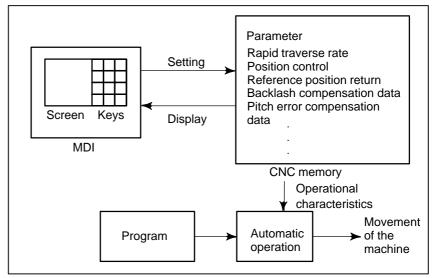
Fig. 1.6 (e) Displaying and setting parameters
