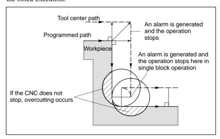
Machining a groove smaller than the tool radius Since the cutter compensation forces the path of the center of the tool to move in the reverse of the programmed direction, overcutting will result. In this case an alarm is displayed and the CNC stops at the start of the block.
