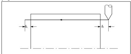
Fig. D.1 (a) Incorrect thread position
