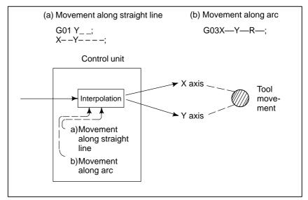
Fig. 1.1 (c) Interpolation function
