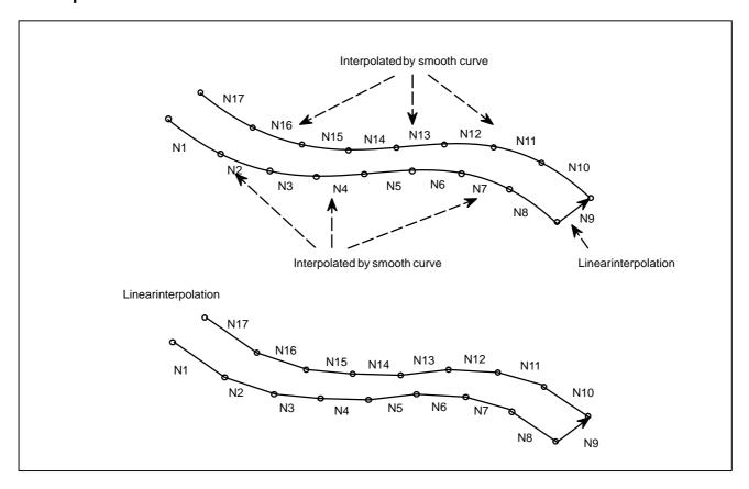
Conditions for performing smooth interpolation Smooth interpolation is performed when all the following conditions are satisfied. If any of the following conditions is not satisfied for a block, that block is executed without smooth interpolation then the conditions are checked for the next block.
