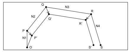
Fig. 22.5.1 (I) When a Rotation Axis and Linear Axis Are Specified at the Same Time
