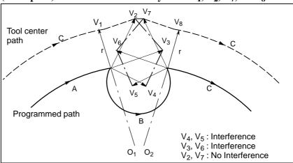
(Example 2) The tool moves linearly from  $V_1$ ,  $V_2$ ,  $V_7$ , to  $V_8$
