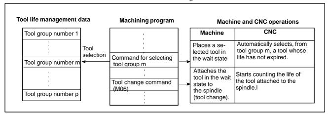
Fig. 10.2 (b) Tool Selection by Machining Program
