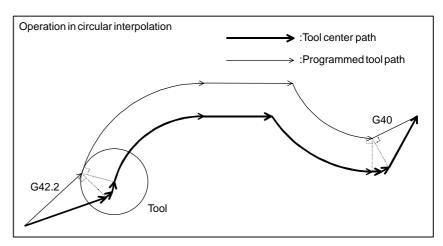
Fig. 22.5.1 (c) Operation at compensation start-up and cancellation (Type B)
