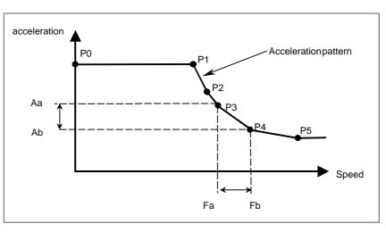
Fig.19.10 (c) Setting acceleration pattern
