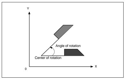
Fig. 14.10 (a) Coordinate system rotation
