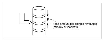
Fig. 5.3 (c) Feed per revolution
