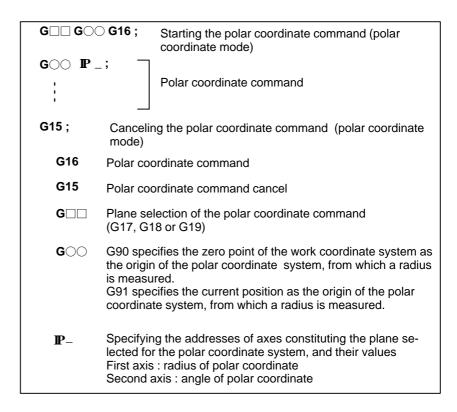
Setting the zero point of the workpiece coordinate system as the origin of the polar coordinate system Specify the radius (the distance between the zero point and the point) to be programmed with an absolute command. The zero point of the work coordinate system is set as the origin of the polar coordinate system. When a local coordinate system (G52) is used, the origin of the local coordinate system becomes the center of the polar coordinates.
