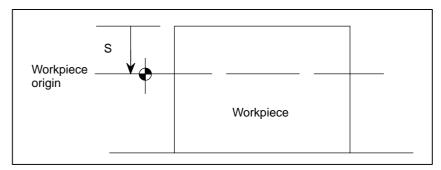
**8** To measure any subsequent workpiece origins, retract the tool from the workpiece, then repeat steps 5 to 7.
