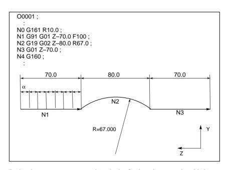
In the above program, every time the in–feed cutting start signal is input, the tool is moved by 10.000 along the machining profile shown above.  $\alpha$ = Travel distance for each in–feed control cutting start signal input The feedrate is programmed with an F code.
