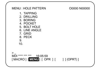
3 Enter a pattern number and press soft key [SELECT]. In this example, press 5, then press [SELECT]. The following screen (pattern data screen) is displayed:
