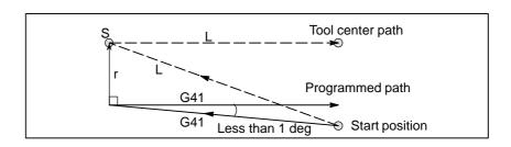
A block without tool movement specified at start-up If the command is specified at start-up, the offset vector is not created.
