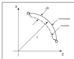
$$\Delta r = \frac{1}{2} (T_1^2 + T_2^2 (1 - \alpha^2)) \frac{V^2}{r} \dots (1)$$
