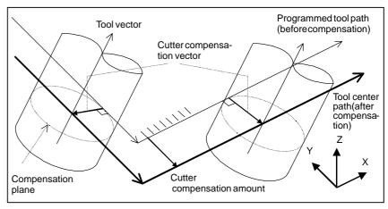
Fig. 22.5.1 (a) Tool side compensation
