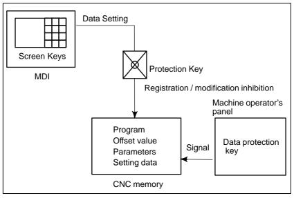
Fig. 1.6 (f) Data Protection Key
