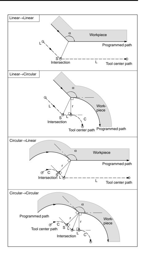
Tool movement around the outside corner at an acute angle (α<90°)</li>
