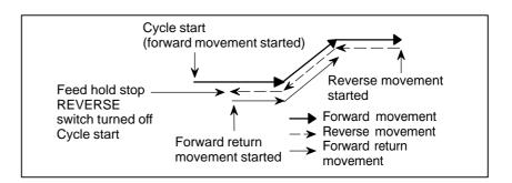
Reverse movement → Reverse movement completion → Forward return movement When there are no more blocks for which to perform reverse movement (when the tool has moved back to the initial forward movement block or the tool has not yet started forward movement), the reverse movement completion state is entered and operation stops.
