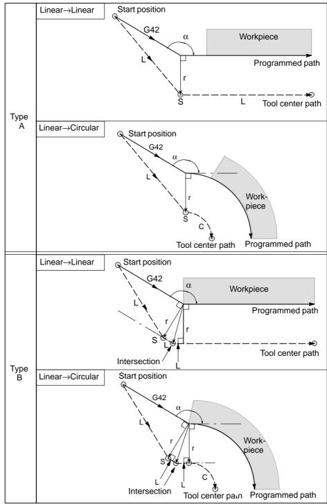
Tool movement around the outside of an acute angle (α<90°)</li> Tool path in start—up has two types A and B, and they are selected by parameter SUP (No.5003#0).
