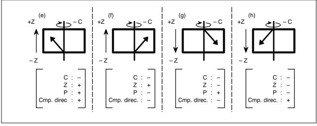
Fig. 20.8.3 (c) Direction of helical gear compensation
