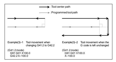
Fig. 22.5.1 (h) Operation in the compensation mode (3)
