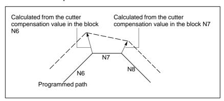
Fig. 14.5 (c) Changing the Cutter Compensation Value
