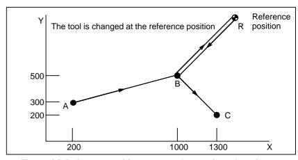
Fig. 6.1 (c) Reference position return and return from the reference position
