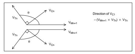
Fig. 22.5.2 (h) Direction of the compensation vector (2)
