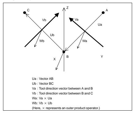
Fig. 22.5.1 (q) Conceptual Diagram
