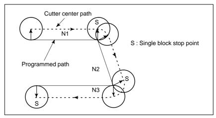
Fig. 14.11 (e) Point at which a Single–Block Stop Occurs in the Normal Direction Control Mode
