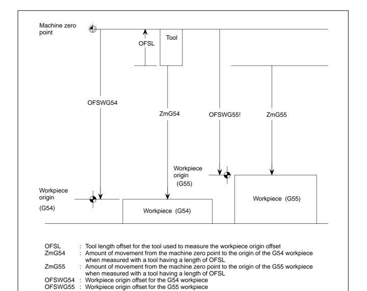
As can be seen from the above figure, the Z-axis workpiece origin offset can be calculated from the following formula:
