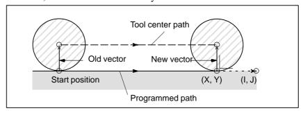
In case the old vector is 0, this command specifies the equipment to enter from the cancel mode into the cutter compensation mode. At this time, the offset number is specified by the H code.
