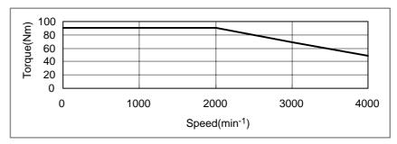
Fig.19.10 (e) Torque for Acc/Dec with consideration of friction
