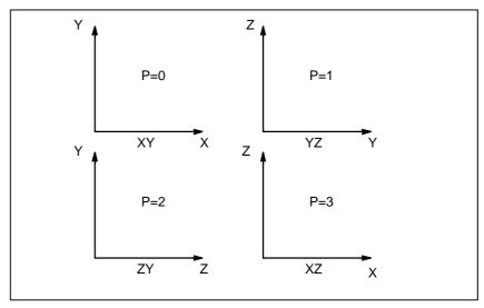
Fig. 12.1(e) Coordinate systems for the plane view
