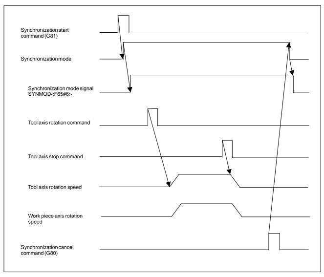
Fig. 20.8.3 (b) Example timing for starting/canceling synchronization
