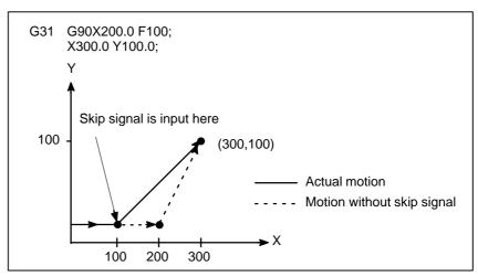
Fig 4.16 (c) The next block is an absolute command for 2 axes
