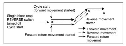
In the case of 3) above, the tool starts forward return movement at the position of a feed hold stop when the cycle start switch is pressed.
