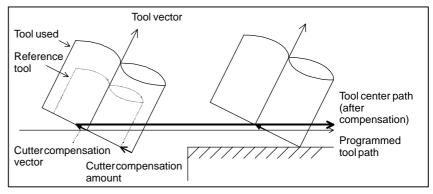
Fig. 22.5.2 (a) Reading edge offset
