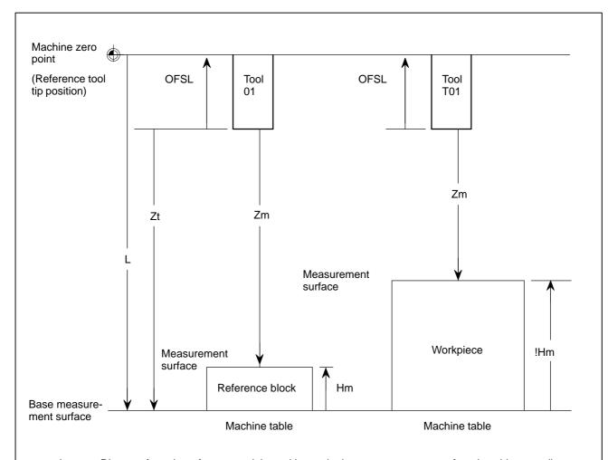
$L \qquad : \ \, \text{Distance from the reference tool tip position to the base measurement surface (machine coordinate} \\$
