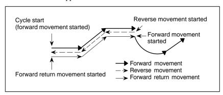
If the tool moves in the reverse direction after a feed hold stop, the tool stops forward return movement at the position of the feed hold stop, then resumes forward movement. If the tool moves in the reverse direction after a single block stop, the tool also stops forward return movement at the position of the single block stop.
