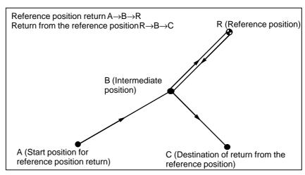
Fig. 6.1 (b) Reference position return and return form the reference position
