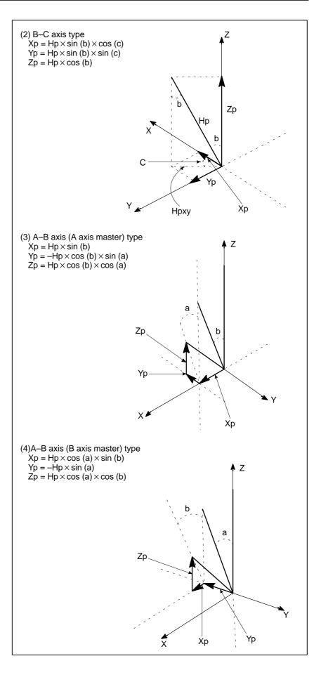
In the figures above, a, b, and c represent the positions (angles) of the A-axis, B-axis, and C-axis from the machine zero point; those values present when the tool axis direction handle feed mode is set or a reset occurs are used. To change the feed direction, reenter the tool axis direction handle feed mode, or press the reset key.
