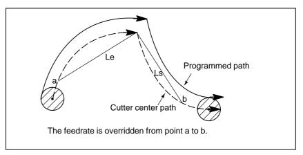
Fig. 5.4.2.1 (c) Override Range (Arc to Arc)
