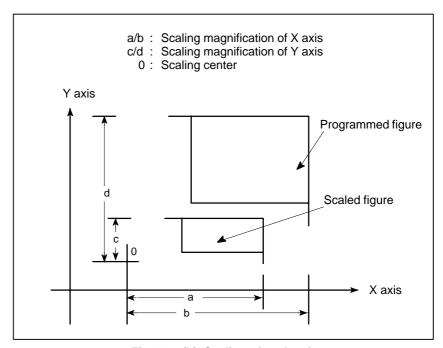
Fig. 14.9 (b) Scaling of each axis
