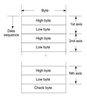
In the data format for binary input operation, the travel distance along each axis (2 bytes) per unit time is specified. The travel distances along all axes are placed sequentially from the first axis, then a check byte is added. (The data length for one block is [2 x N + 1] bytes).
