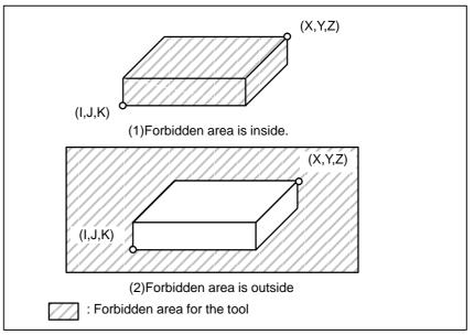
Fig. 6.3 (a) Stroke check
