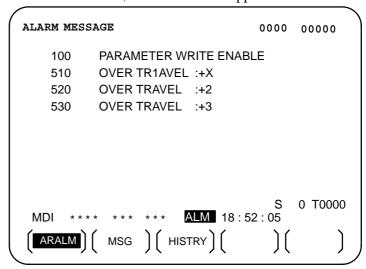
Another method for alarm displays In some cases, the alarm screen does not appear, but an ALM is displayed at the bottom of the screen.
