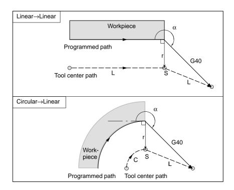
Tool movement around an outside corner at an obtuse angle (90° ≤ α<180°)</li> Tool path has two types, A and B; and they are selected by parameter SUP (No. 5003#0).
