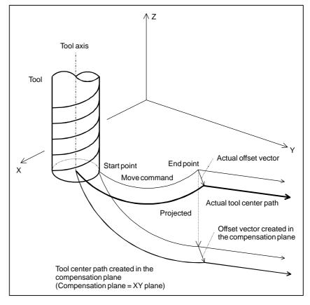
Fig. 22.5.1 (i) Operation in the compensation mode (4)
