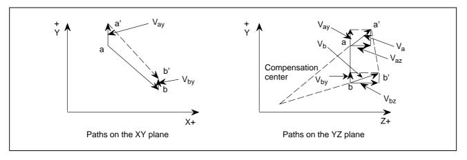
(Example 2) When the compensation axes are the Y- and Z-axes and circular interpolation is performed for the X- and Y-axes Programmed path:  $a \rightarrow b$ , compensated path:  $a' \rightarrow b'$
