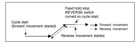
Reverse movement → Forward return movement Three methods are available for moving the tool in the forward direction again along the retraced path.
