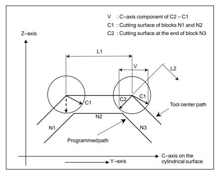
Fig. 22.2 (f) When the Amount of Travel (L1) of Block N2 Is Less Than the Parameter Value
