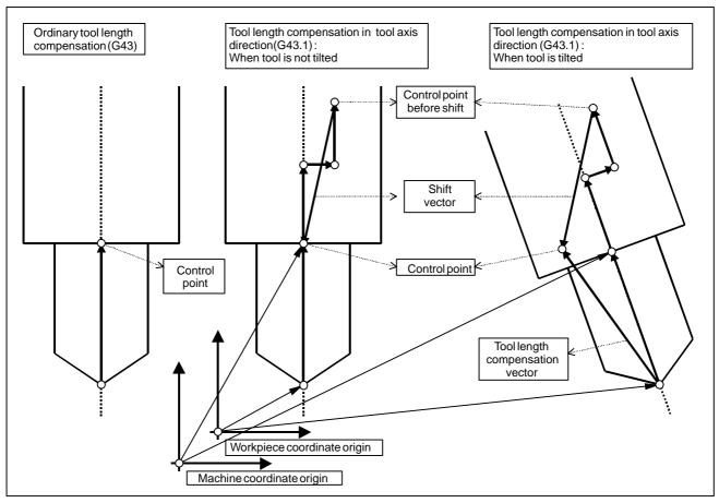
Fig. 22.4 (e) Shift of the Control Point
