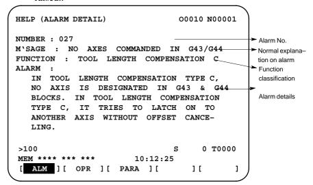
Fig. 13 (b) ALARM DETAIL Screen when P/S Alarm No. 27 is issued
