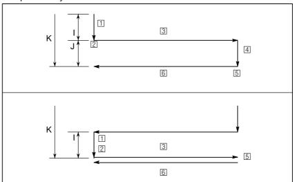
Chart of operation in which the total depth of cut is reached during cutting specified by I and J:
