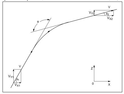
Fig. D.3 (b) Example of tool path
