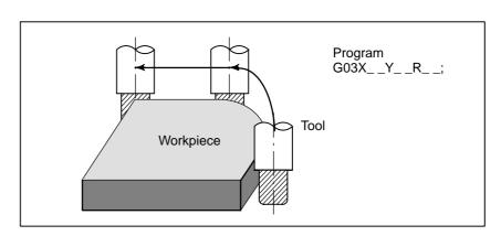
Fig. 1.1 (b) Tool movement along an arc
