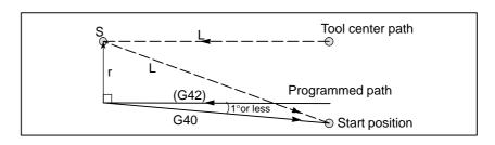
When a block without tool movement is commanded together with an offset cancel, a vector whose length is equal to the offset value is produced in a normal direction to tool motion in the earlier block, the vector is cancelled in the next move command.
