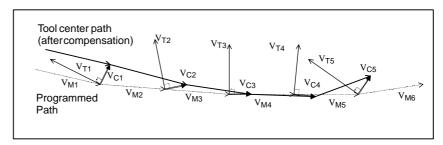
Fig. 22.5.2 (o) When  $\theta$ =90deg. Is Determined (2)
