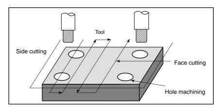
Prepare the program of the tool path and machining condition according to the workpiece figure, for each machining.
