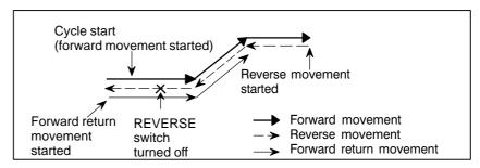
In the case of 2) above, the tool starts forward return movement at the position of a single block stop when the cycle start switch is pressed.
