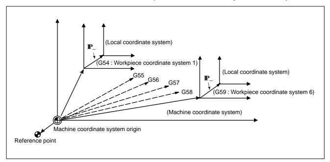
Fig. 7.3 Setting the local coordinate system
