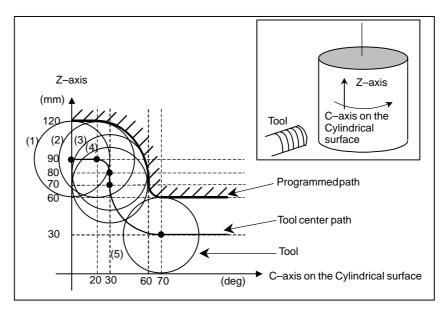
Fig. 22.2 (j) Path of Sample Program for Cylindrical Interpolation Cutting Point Compensation
