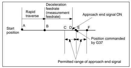
Fig. 14.2 (b) Tool movement to the measurement position
