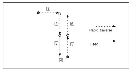
Fig. 5.5 (b) Single block during canned cycle
