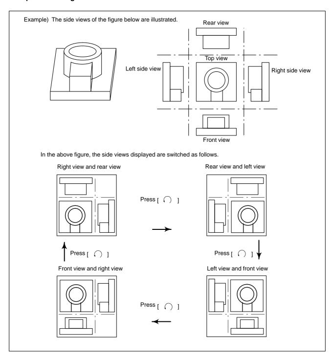
Cross section position selection in triplane drawing Some examples of cross–sectional views are given below for the left view and front view shown on the previous page.
