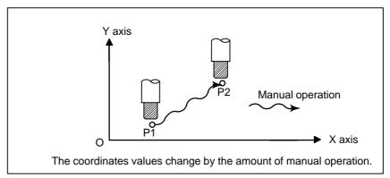
Fig. 3.5 (a) Coordinates with the switch ON
