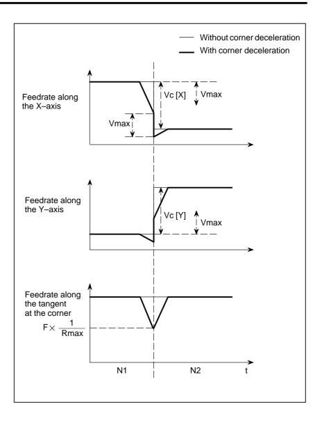
Setting the allowable feedrate difference along each axis
