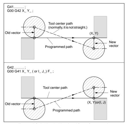
Fig. 14.4.5 Switching the Direction of Cutter Compensation
