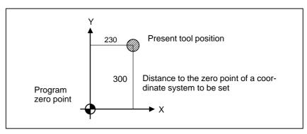
Fig. 1.3.2 (b) Coordinate system specified by the CNC
