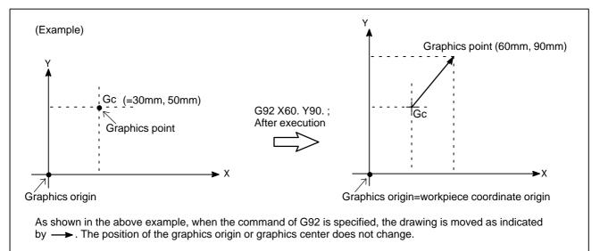
Fig. 12.1 (c) Workpiece coordinate origin and graphics origin
