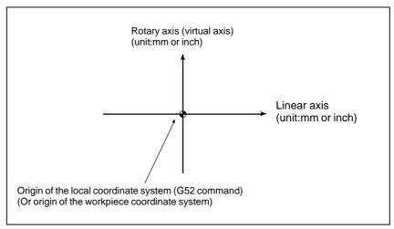
Fig. 4.8 (a) Polar coordinate interpolation plane.
