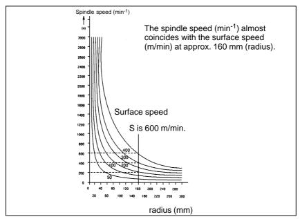
Fig. 9.3 (a) Relation between workpiece radius, spindle speed and surface speed
