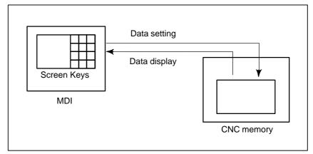
Fig. 1.6 (a) Displaying and Setting Data
