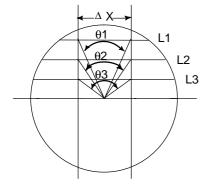
Consider lines L1, L2, and L3.  $\Delta X$  is the distance the tool moves per time unit at the feedrate specified with address F in the Cartesian coordinate system. As the tool moves from L1 to L2 to L3, the angle at which the tool moves per time unit corresponding to  $\Delta X$  in the Cartesian coordinate system increases from $\theta 1$  to  $\theta 2$  to  $\theta 3$ .
