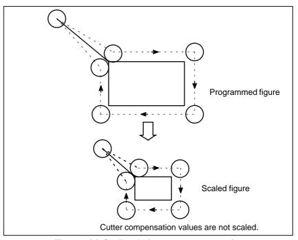
Fig. 14.9 (e) Scaling during cutter compensation
