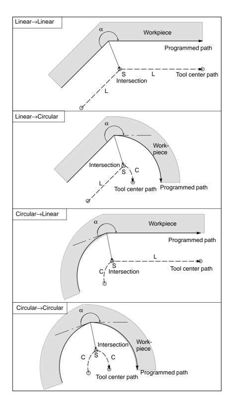
• Tool movement around the inside ( $\alpha$ <1°) with an abnormally long vector, linear  $\rightarrow$  linear
