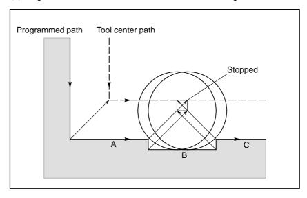
There is no actual interference, but since the direction programmed in block B is opposite to that of the path after cutter compensation the tool stops and an alarm is displayed.
