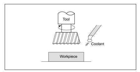
The function of specifying the on–off operations of the components of the machine is called the miscellaneous function. In general, the function is specified by an M code (See II–11).
