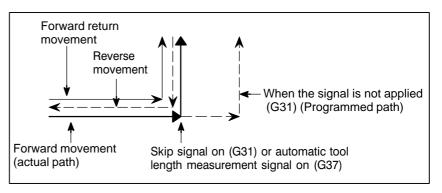
Chopping function (G81.1) Whether the chopping operation is performed in reverse movement and forward return movement is determined by whether the chopping operation was performed at the end of forward movement.
