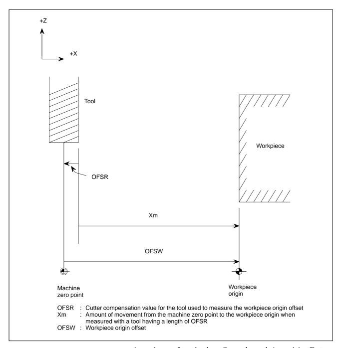
As can be seen from the above figure, the workpiece origin offset can be calculated from the following formula:
