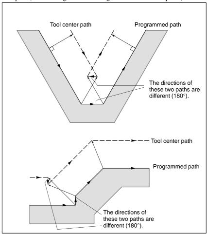
(2) In addition to the condition (1), the angle between the start point and end point on the tool center path is quite different from that between the start point and end point on the programmed path in circular machining (more than 180 degrees).
