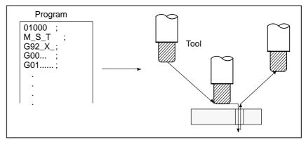
Fig. 1.2 (a) Tool Movement by Programming
