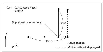
Fig. 4.16 (a) The next block is an incremental command
