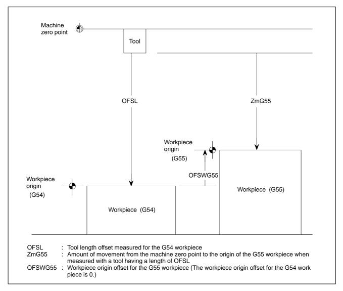
For definition 2, the workpiece origin offset can be calculated using the same formula as that used for definition 1:
