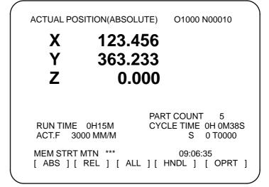
Fig. 2.5.1 Position screen (Seven soft key type)
