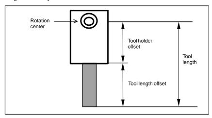
Fig. 22.4 (b) Tool Holder Offset
