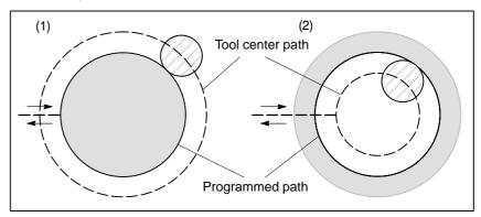
Fig. 14.5 (d) Tool Center Paths when Positive and Negative Cutter Compensation Values are Specified
