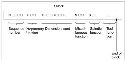
Fig. 1.7 (b) Block configuration
