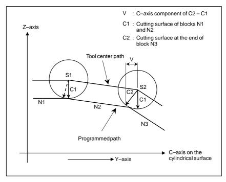
Fig. 22.2 (e) When Bit 6 (CYS) of Parameter No. 6004 Is 0
