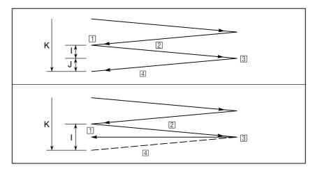
Chart of operation in which the total depth of cut is reached during cutting specified by I and J:
