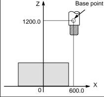
If an absolute command is issued, the base point moves to the commanded position. In order to move the tool tip to the commanded position, the difference from the tool tip to the base point is compensated by tool length offset.
