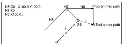
Two blocks without tool movement should not be commanded consecutively. If commanded, a vector whose length is equal to the offset value is produced in a normal direction to tool motion in earlier block, so overcutting may result.
