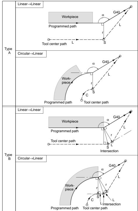
Tool movement around an outside corner at an acute angle (α<90°)</li> Tool path has two types, A and B: and they are selected by parameter SUP (No. 5003#0)
