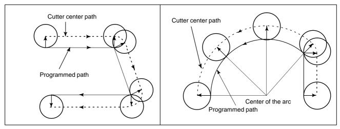
Fig. 14.11 (b) Normal direction control left (G41.1)
