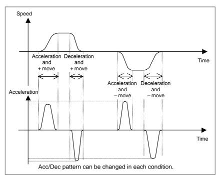
Fig.19.10 (b) Acceleration/deceleration with this function
