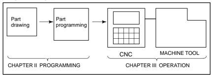
Before the actual programming, make the machining plan for how to machine the part.
