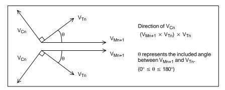
Fig. 22.5.2 (g) Direction of the compensation vector (1)
