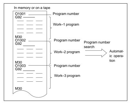
Fig. 1.3 (a) Program Selection for Automatic Operation
