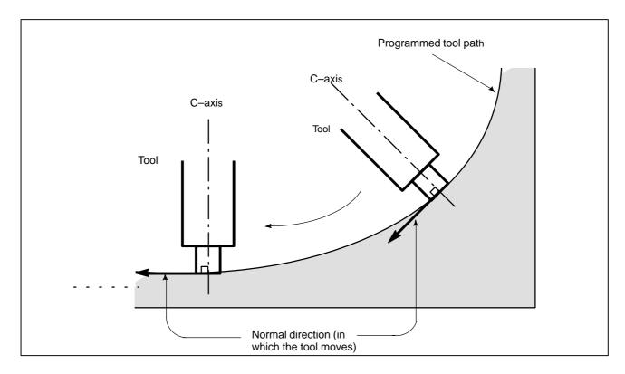
Fig. 14.11 (a) Sample Movement of the tool
