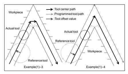
Fig. 22.5.1 (f) Operation in the compensation mode (1)-3, 4
