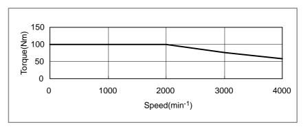
Fig.19.10 (d) Speed–torque characteristics of model  $\alpha$ 30/4000i
