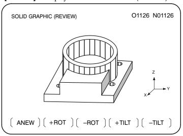
14 Press soft key **[(OPRT)]**, then press soft key **[ANEW]**. The machining figure is redrawn with the color, intensity, or drawing direction set in **step 13**.
