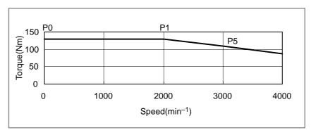
Fig.19.10(i) Torque for Acc/Dec in case of + move and deceleration
