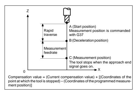
Fig. 14.2 (a) Automatic tool length measurement
