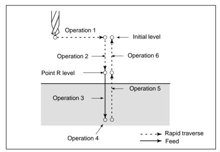
Fig. 13.1 Canned cycle operation sequence
