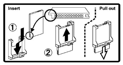
3) Assembling of the attachment Insert the memory card with the attachment into the memory card interface as following figure. And, fix the attachment guide by screwing the screw of the attachment guide by manual.
