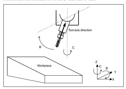
Fig. 22.4 (a) Tool Length Compensation in Tool Axis Direction
