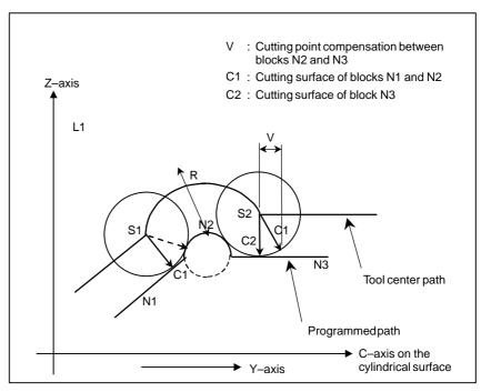
Fig. 22.2 (g) When the Diameter of an Arc Is Less Than the Parameter Value
