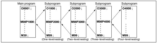
A single call command can repeatedly call a subprogram up to 999 times. For compatibility with automatic programming systems, in the first block, Nxxxx can be used instead of a subprogram number that follows O(or:). A sequence number after N is registered as a subprogram number.
