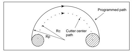
Fig. 5.4.2.2 Internal circular cutting feedrate change
