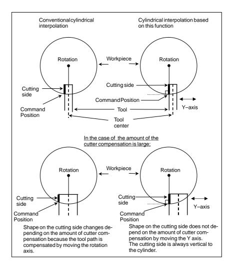
Fig. 22.2 (a) Comparison with Conventional Interpolation
