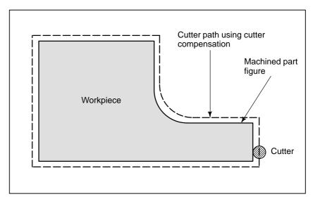
If radius of cutters are stored in the CNC (Data Display and Setting : see III–11), the tool can be moved by cutter radius apart from the machining part figure. This function is called cutter compensation.
