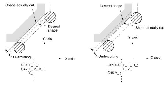
2 G45 to G48 (tool offset) must not be used in the G41 or G42 (cutter compensation) mode.
