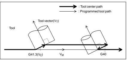
Fig. 22.5.2 (c) When the tool vector is inclined in the direction opposite to the direction the tool moves
