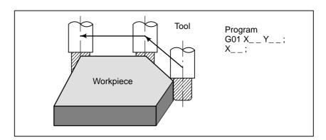
Fig. 1.1 (a) Tool movement along a straight line
