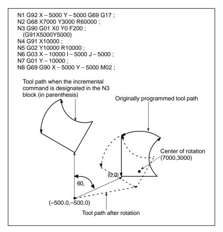
Fig. 14.10 (c) Absolute/incremental command during coordinate system rotation
