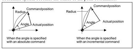
Setting the current position as the origin of the polar coordinate system Specify the radius (the distance between the current position and the point) to be programmed with an incremental command. The current position is set as the origin of the polar coordinate system.
