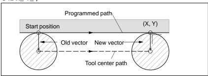
In the case of G00, however, each axis moves independently at the rapid traverse rate.
