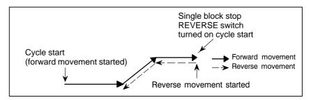
In the case of 3) above, the tool starts reverse movement at the position of a feed hold stop when the cycle start switch is pressed.
