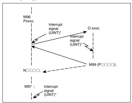
Fig 15.11 Interruption type sustom macro function
