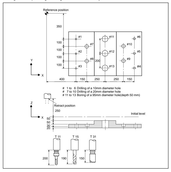
Offset value +200.0 is set in offset No.11, +190.0 is set in offset No.15, and +150.0 is set in offset No.31
