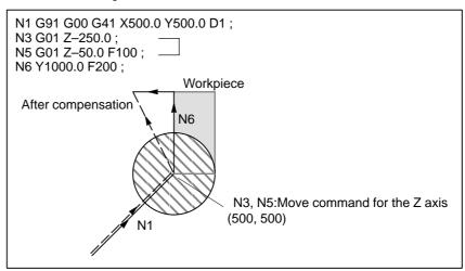
The move command in the same direction as that of the move command after the motion in Z axis should be programmed.
